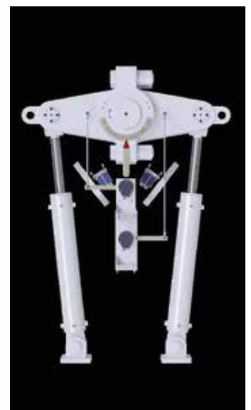
DMC - Piston-type steering gear.
