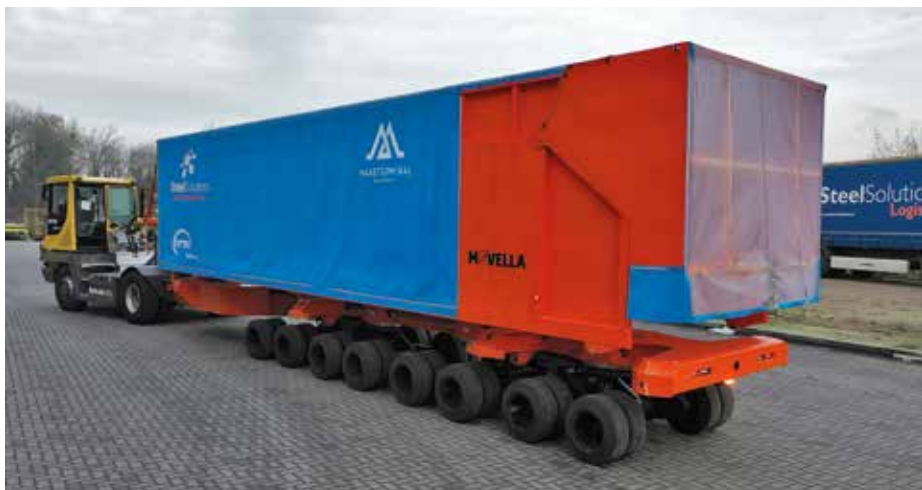
Terberg terminaltrekker met unieke custom made transliifter.
